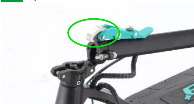
4 Once the main lever is released, ensure that the capture is also released
